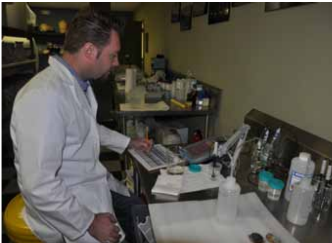
Fig. 2. Odyssey's chief conservator Fred van de Walle recording levels of chloride ion extraction within sodium sesquicarbonate solution using a Fisher Scientific Accumet XL50 meter.
