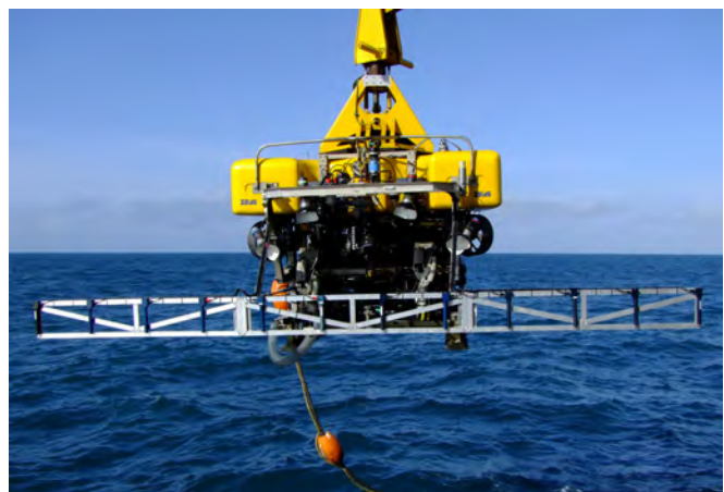
Fig. 2. FADE equipment wings extended in front of the ROV Zeus in preparation for survey.
