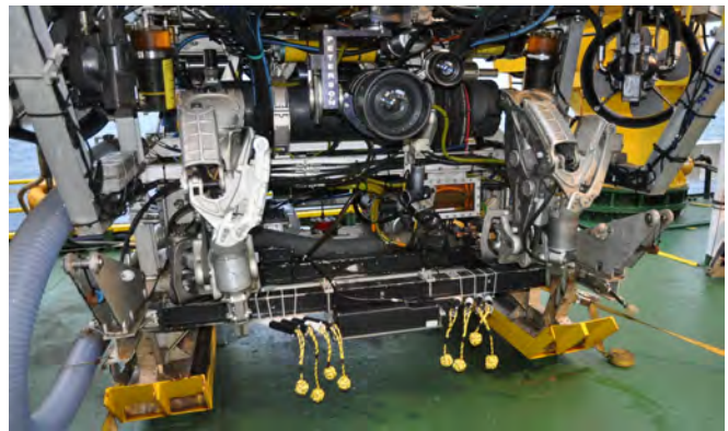
Fig. 1. Multibeam transducers mounted on the ROV Zeus.
