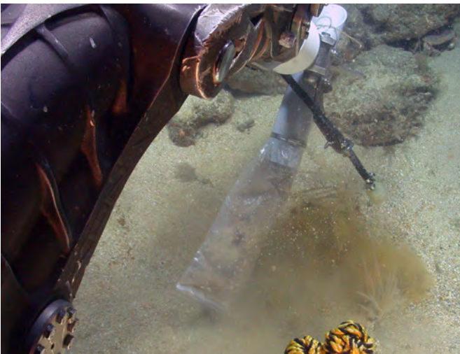
Figs. 54-55. Sediments being sampled from the top stratum of Area F (Phase 2 non-disturbance site survey).
